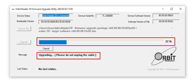
12. Do not unplug the cable. Wait for the message "Device upgrade has been completed" on the upgrade utility or until the Orbit Reader 20 reboots and shuts down.
