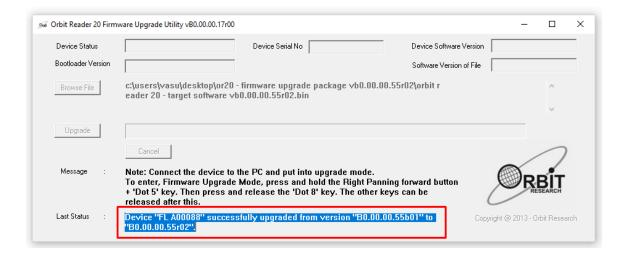
13. The Orbit Reader 20 is upgraded. Turn on to start using the device.
